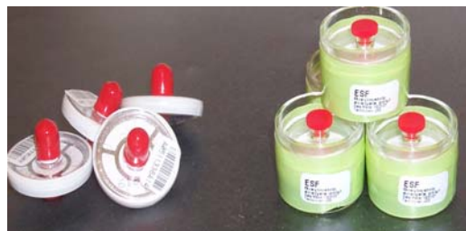
Wood Dust Saucer Cassette (left) ESF Gravimetric Only Cassette (right)
