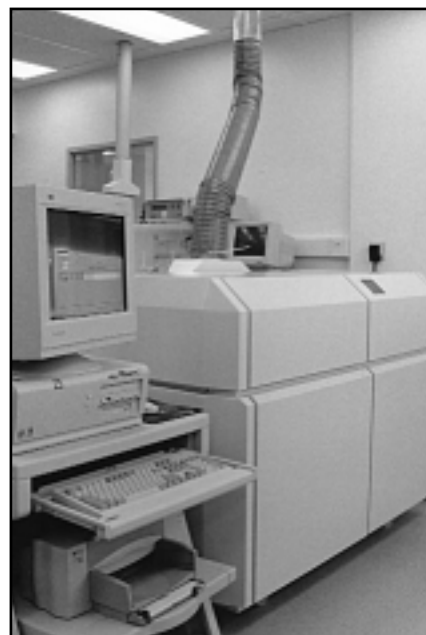
The new ICP Mass Spectrometer is located in the Trace Metals Clean Room.
