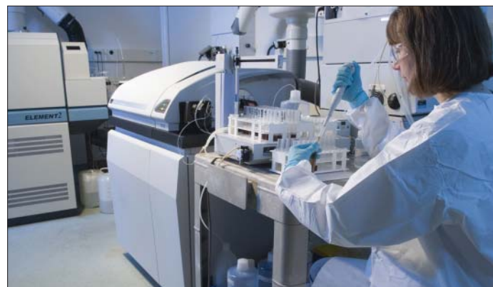
In the Trace Element Clean Laboratory, a WSLH chemist prepares to analyze samples on an inductively coupled plasma-mass spectrometer (ICP-MS), which can test clinical and environmental samples for a variety of elements, including toxic metals at very low levels. In the background is an inductively coupled plasma-high resolution mass spectrometer (HR-ICP-MS) that can further resolve individual isotopes of elements at extremely low concentrations.
