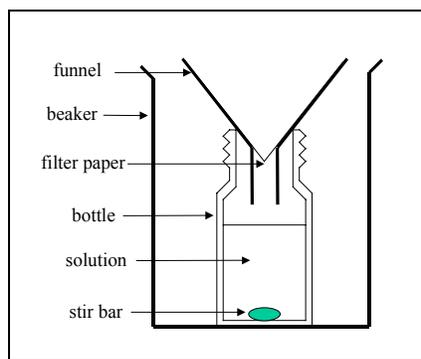
Figure 1. Filter Setup.
