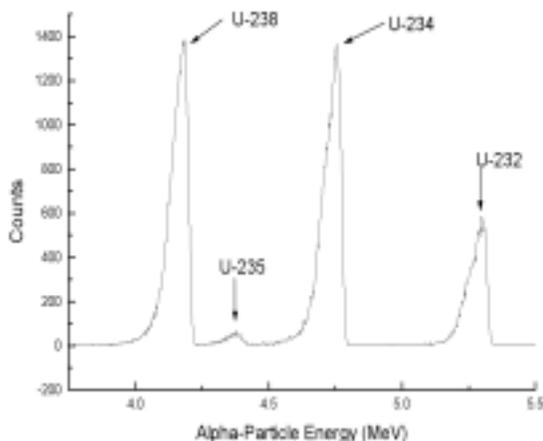
**Figure 2.** Spectrum of Uranium Proficiency Standard.
