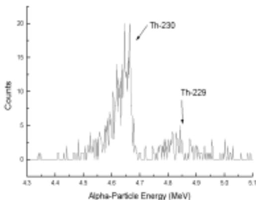
**Figure 4.** Alpha-particle spectrum of proficiency standard after column funnel had been cleaned.
