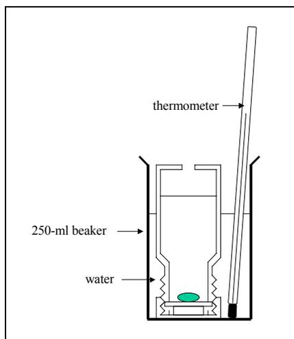
Figure 3. Schematic of Hot Water Bath.
