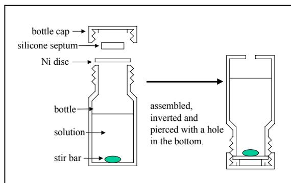
Figure 2. Schematic of Deposition Cell.
