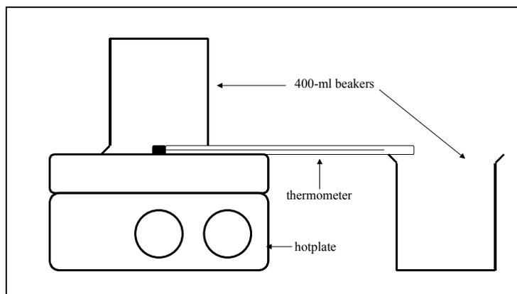
Figure 4. Heating Apparatus for Oxidizing Polonium on Ni disc.
