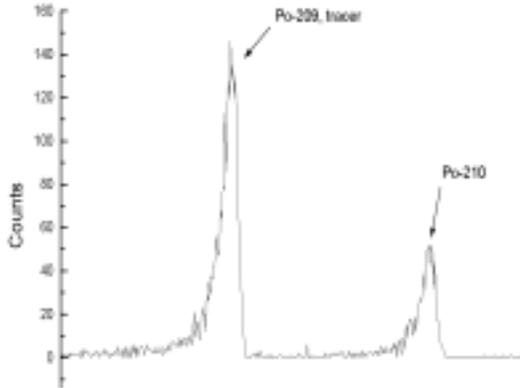
**Figure 1.** Plot of Polonium Spectrum for a 10-L sample of Madison tap water.
