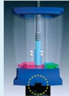
4. Sonic horn breaks up organisms and releases DNA
